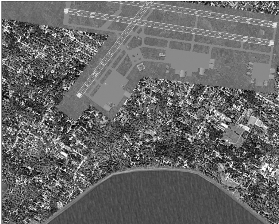
Figure 6-2: A reasonably “attractive” satellite image. The raw screenshot was cropped to 8x10. In Photo Shop Image>Mode>Grayscale was selected. Then Image>Adjustments>Brightness and Contrast and then the sliders adjusted to my liking. You can also add type and filter the image for noise and blurring.
