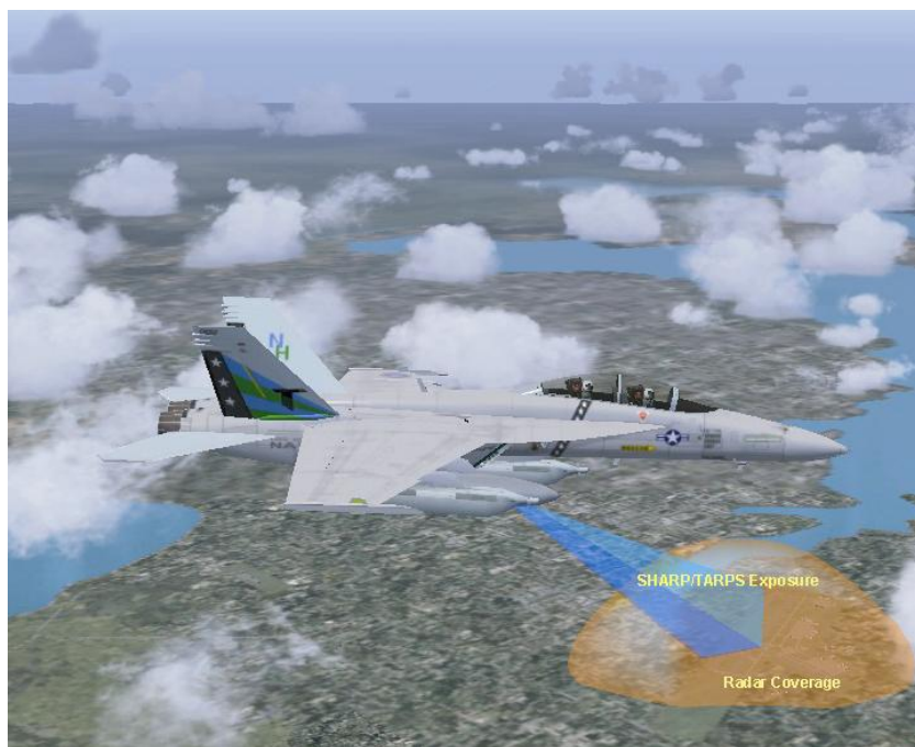
Figure 5-3: Showing flying outside of coverage area at altitude. The exposure is utilizing an oblique angle to cover the area of interest.
