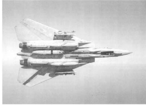
Figure 2-4: Close-up of TARPS and F-14 flying with TARPS.
